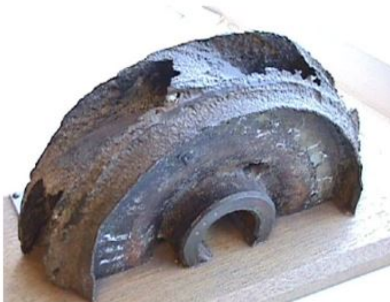
Figure 2. Cavitation damage to an impeller
